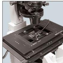
S170C in a Microscope Slide Holder
